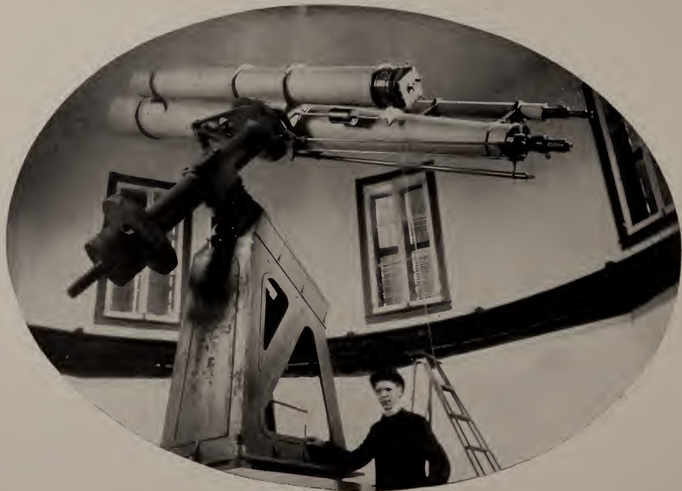
THE TWIN EQUATORIAL TELESCOPE. Visual, 15 inch, Photographic 9 inch aperture.
