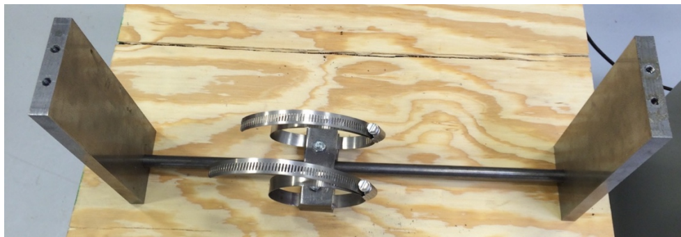
Figure 12: Slider Subassembly Sitting Upside Down
