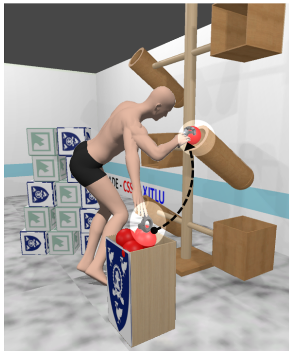
Figure 1. A screenshot of the task based VR environment. The environment was designed to elicit task based movements of users that allowed for biometric identification. Participants would perform movements that were primitively elliptical. In the above example, the user needed to relocate the ball from the bin to the container.
