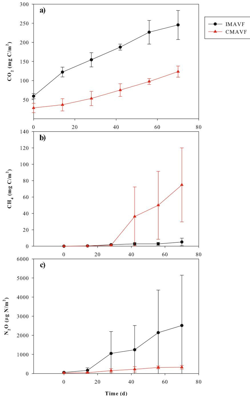
**Fig. 4 Intermittent feeding and gaseous emission.** Effect of intermittent feeding on (a) CO<sub>2</sub>, (b) CH<sub>4</sub> and (c) N<sub>2</sub>O emission. IMAVF Intermittently fed macrophyte assisted vermicfiltration, CMAVF Continuously fed macrophyte assisted vermicfiltration; Error bars: standard deviation created using replicated ( $n = 3$ ) set-ups for each experimental condition.
