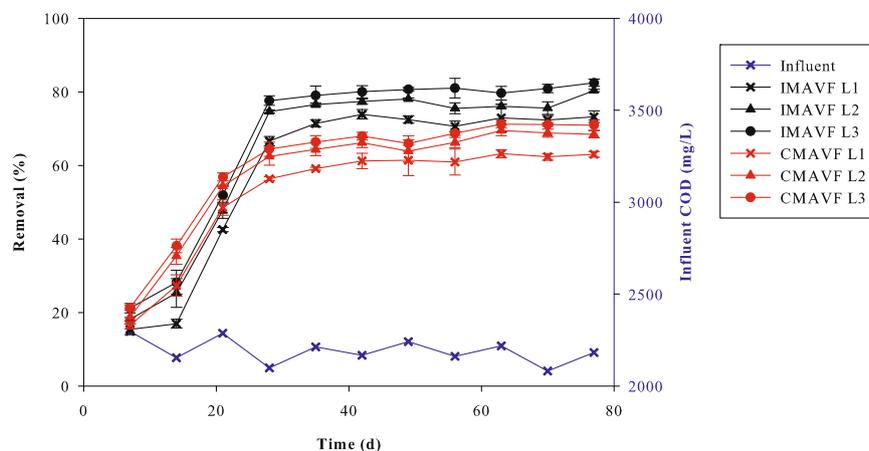
**Fig. 1** Effect of intermittent feeding on COD removal. IMAVF Intermittently fed macrophyte assisted vermifiltration, CMAVF Continuously fed macrophyte assisted vermifiltration; Error bars: standard deviation created using replicated ( $n = 3$ ) set-ups for each experimental condition]. Three layers placed at 0–30 cm (L3), 30–60 cm (L2), and 60–100 cm (L1) from the bottom, containing gravel, alum, and soil mix, respectively.
