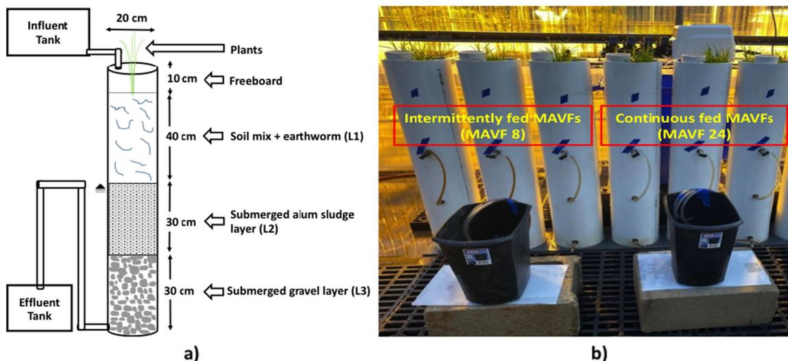
**Fig. 5 Experimental setup.** **a** Schematic. **b** Actual treatment setup. IMAVF [Intermittently fed macrophyte assisted vermifiltration]. CMAVF [Continuously fed macrophyte assisted vermifiltration]. Three layers placed at 0–30 cm (L3), 30–60 cm (L2), and 60–100 cm (L1) from the bottom, containing gravel, alum, and soil mix, respectively.
