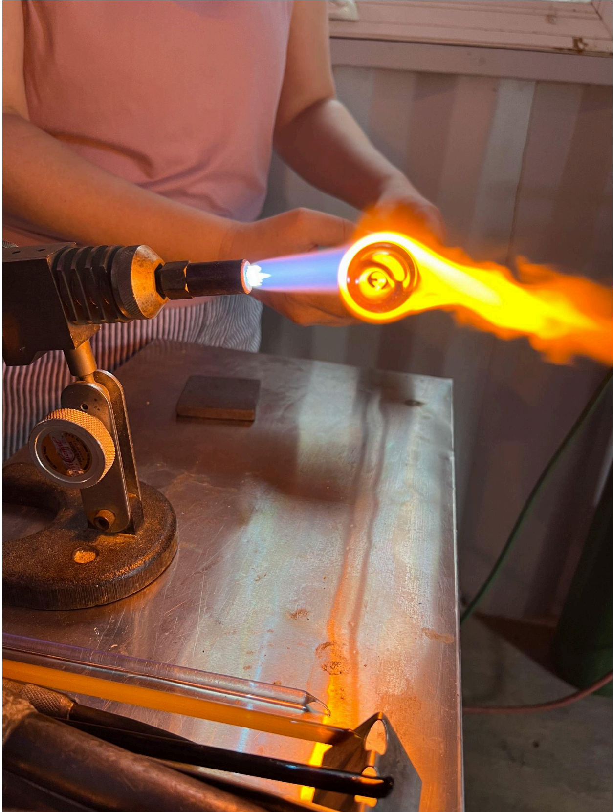
Annealing a glass tube in order to gather glass and blow an ornament
