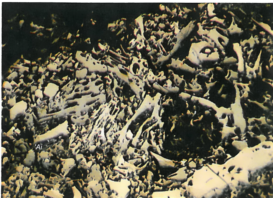
Plate 11: Semifusinite - relatively well-preserved cellular structure and cell walls whose reflecting capacity lies between that of huminite and fusinite. (Photo from seam W-3, magnified 350x.)
