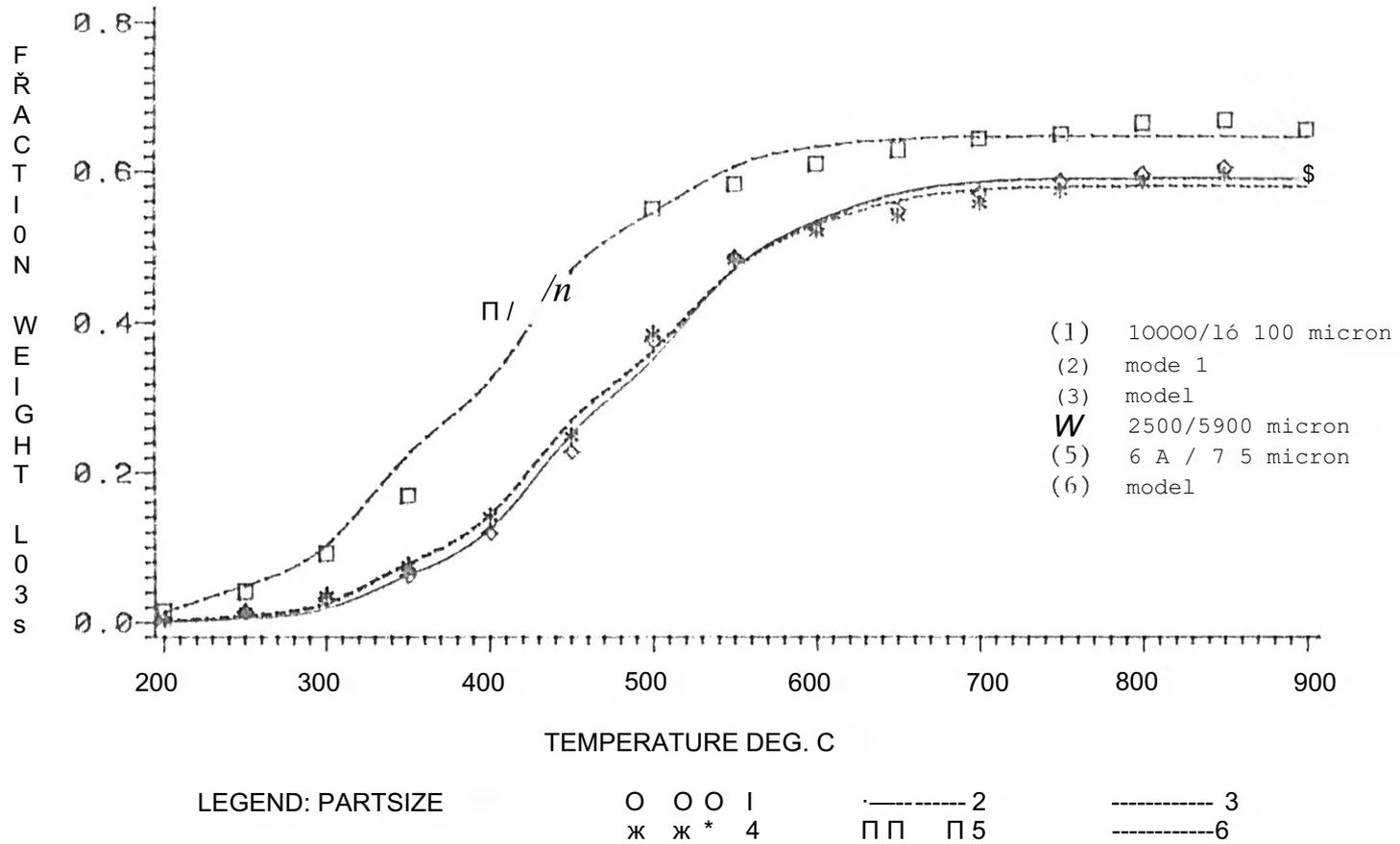
FIGURE 3. EFFECT OF PARTICLE SIZE IN METHANE
