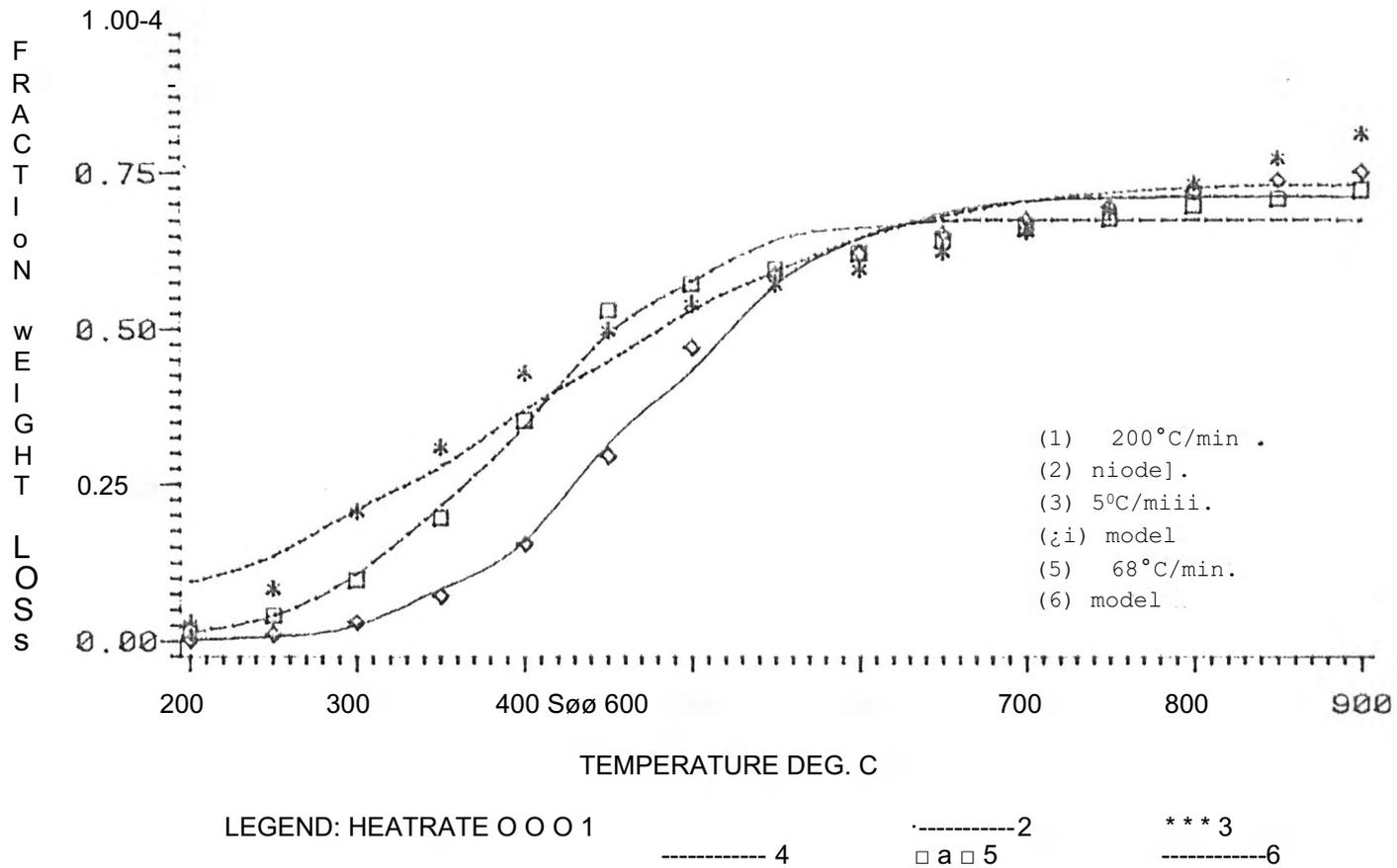
FIGURE 2. EFFECT OF HEATING RATE DEG. C PER MIN. IN HELIUM
