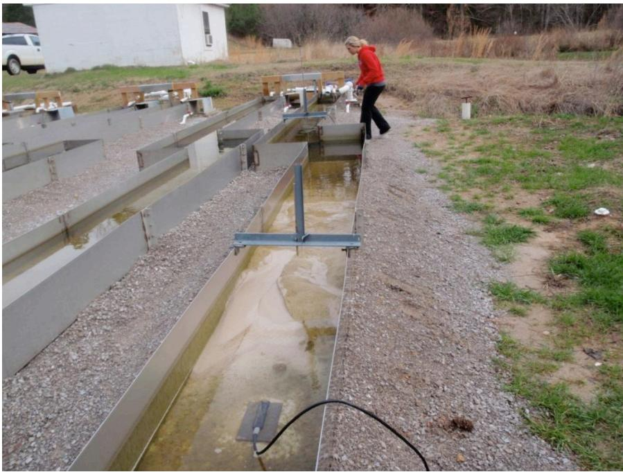
**Figure 3-3: Artificial stream with ~2.5 m sand bed downstream of the pool. The ISCO flowmeter was placed just downstream of the sand bed.**
