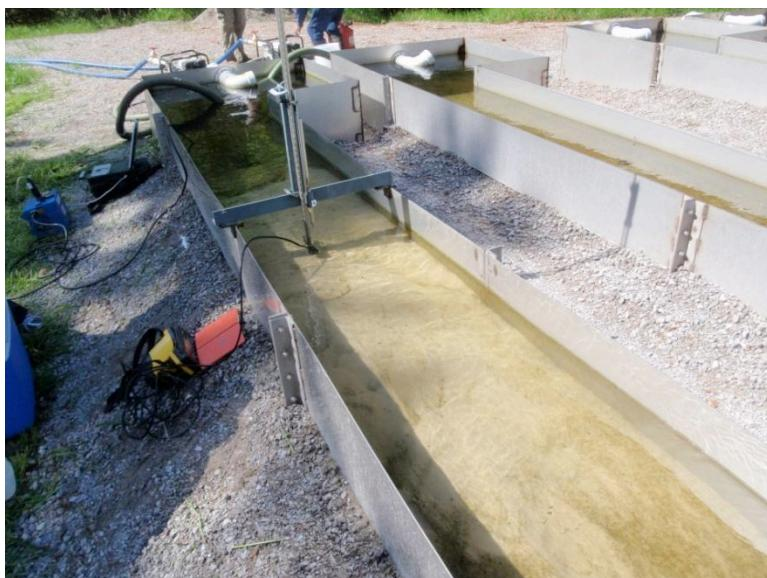
**Figure 3-2: Marsh-McBirney setup and outflow pump location**
