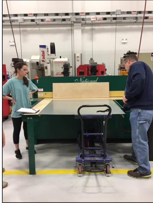
Figure 11: Hydraulic Shear for Cutting Rubber Strips
