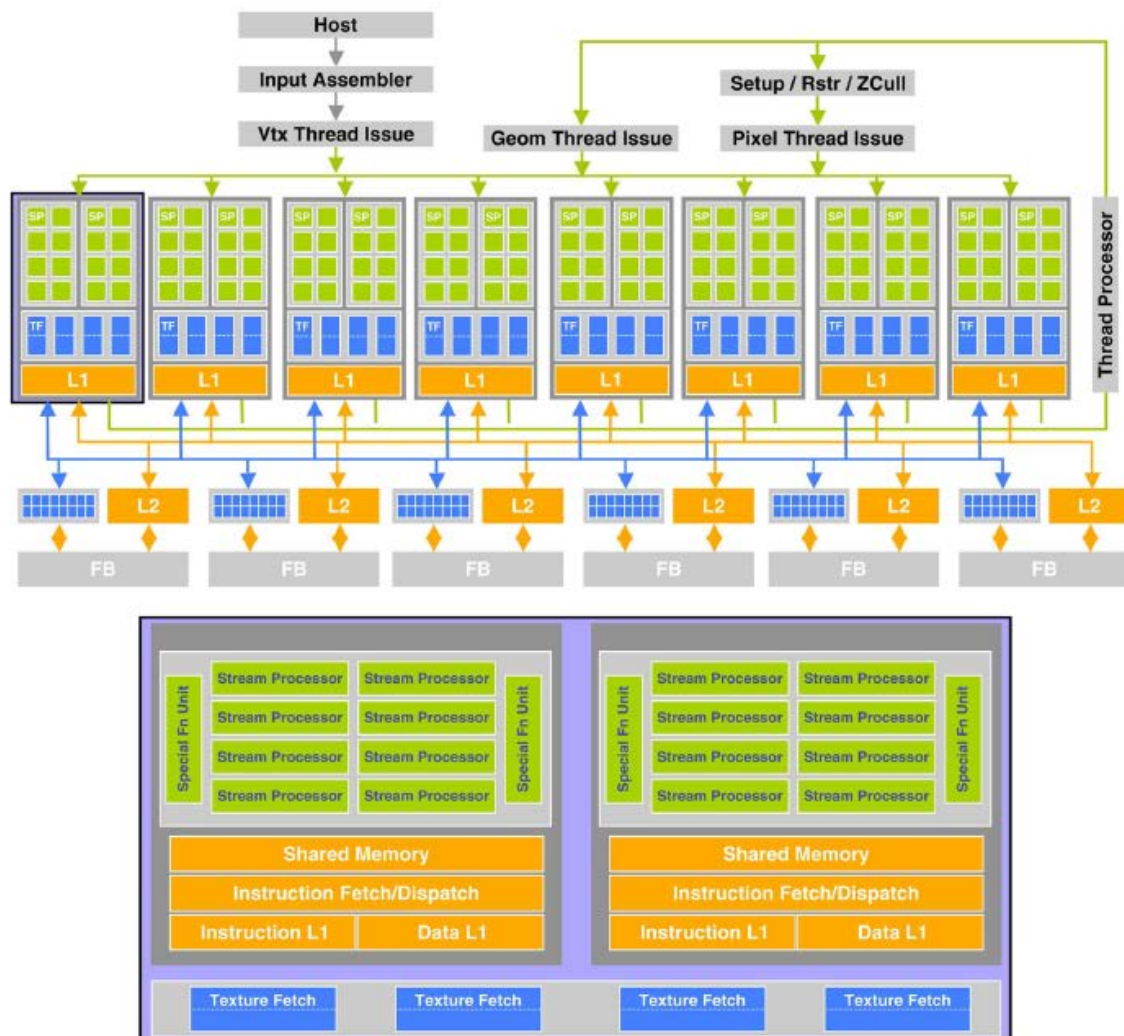
Figure 2.1. NVIDIA GeForce 8800 GTX block diagram. Image courtesy Owens et al[16]
