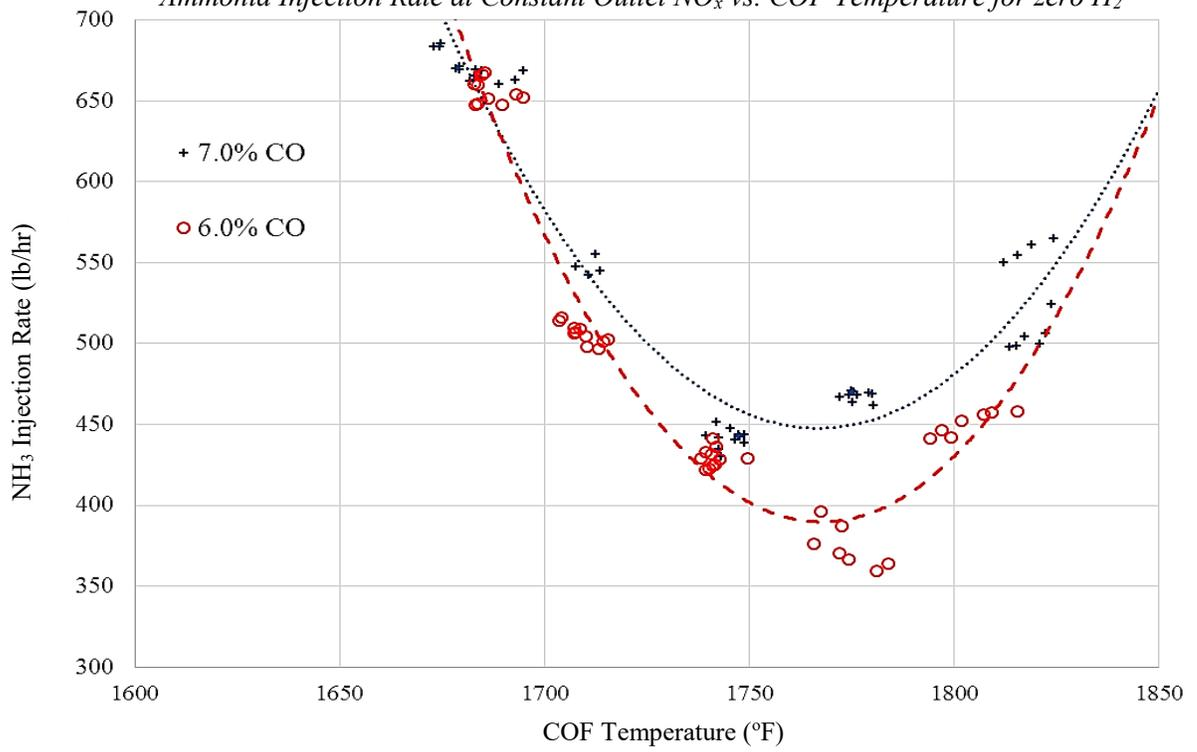
Fig. 7: *Effect of Hydrogen Injection on Thermal DeNO<sub>x</sub> Efficiency: Ammonia Injection Rate at Constant Outlet NO<sub>x</sub> vs. COF Temperature*
