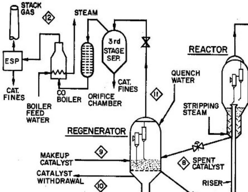
Fig. 3: Regenerator Flue Gas Treatment: General Layout [6]
