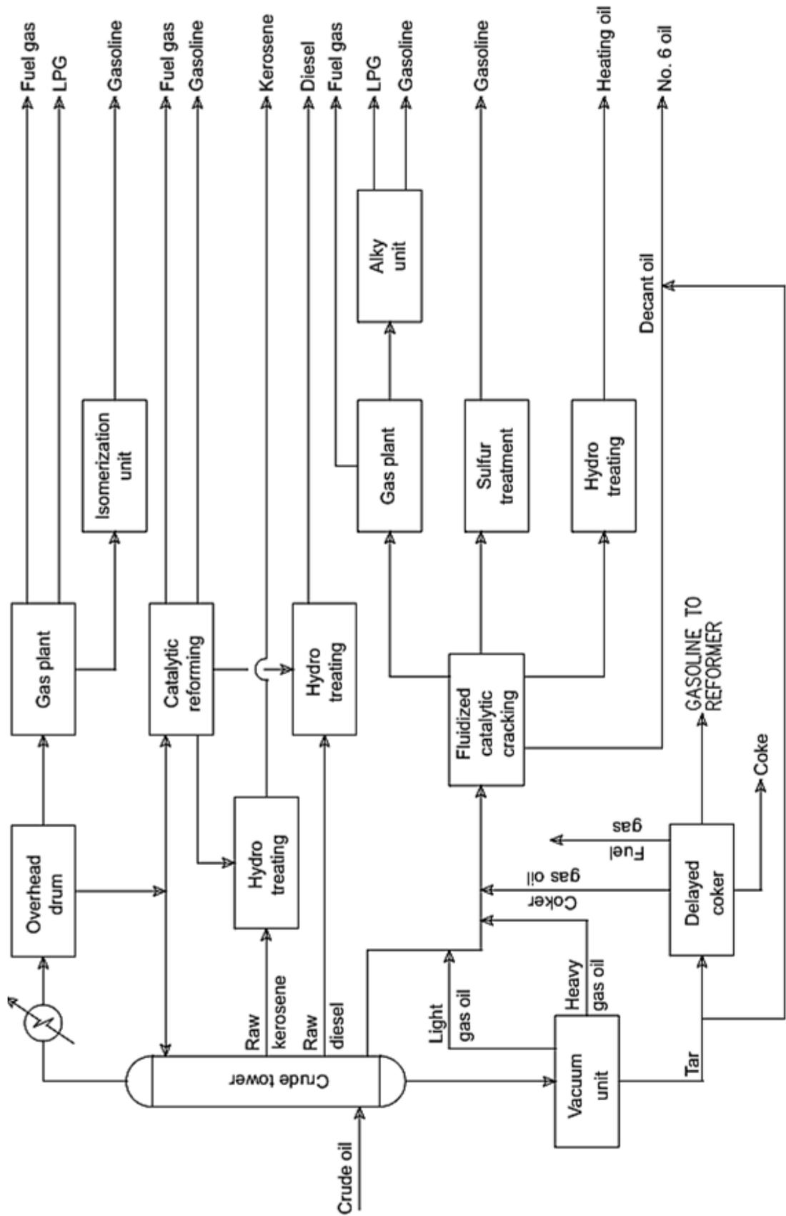
Fig. 1. A Typical High-Conversion Refinery: Simplified Process Flow [4]
