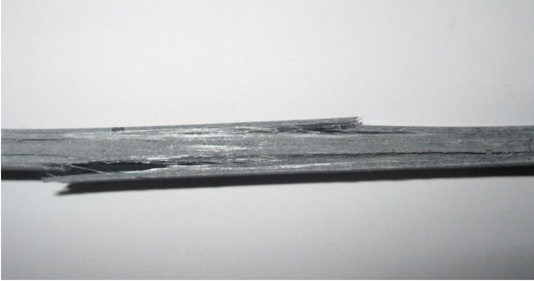
Picture 3. Lateral failure initiated at the lower left location (LGB).
