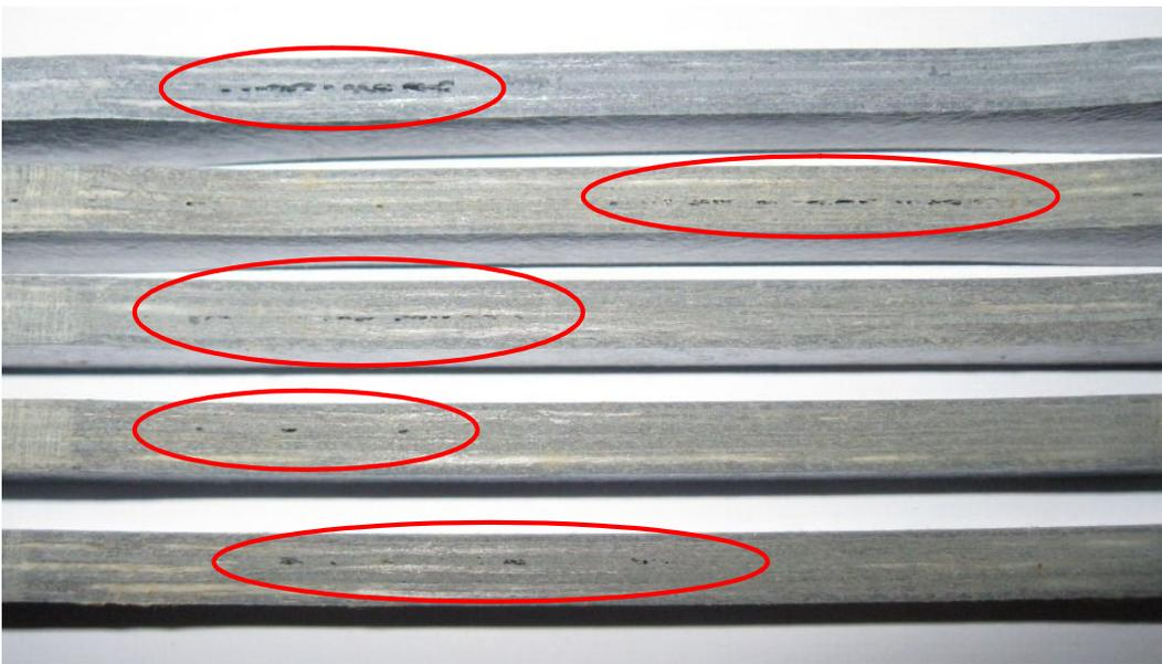
**Figure 6. 30W-samples after 100 FT-cycles**
