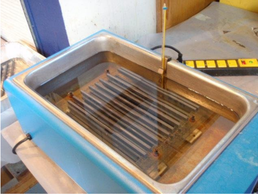
Picture 1. Samples stacked on the rack in a temperature controlled water bath.
