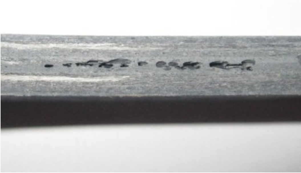
Picture 7. Close-up of 30W-sample after 100 FT-cycles
