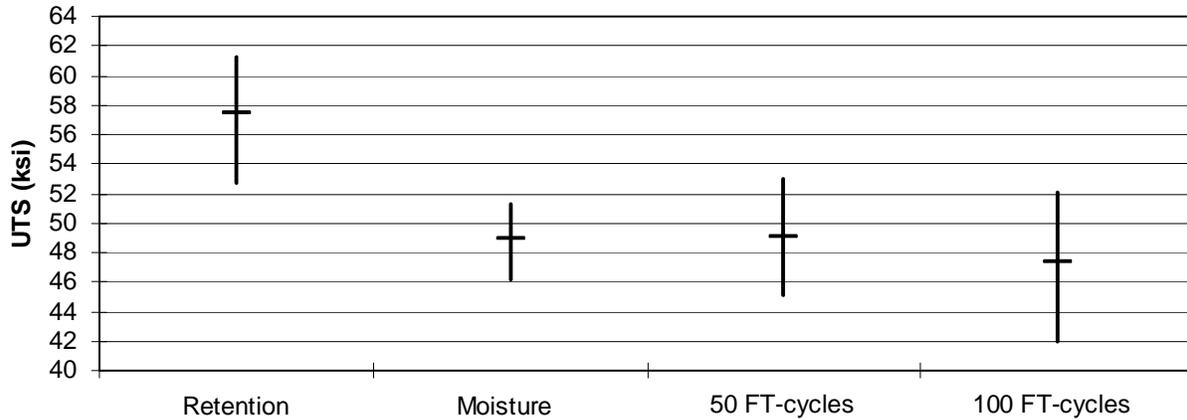
**Figure 7. Progressive UTS display of 60W-samples.**
