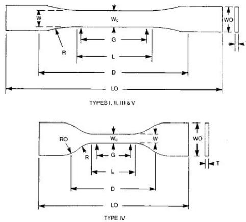
Specimen Dimensions for Thickness,  $T$ , mm [in.]<sup>A</sup>
