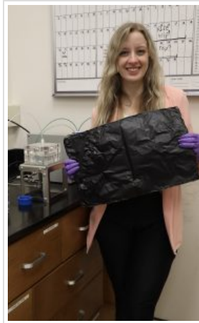
Sarah Grace Zetterholm, a researcher at the U.S. Army Engineer Research and Development Center, displays a graphene mat that can be used as a membrane in water filtration systems or as an adsorbent to pull toxins out of water. Photo courtesy U.S. Army Corps of Engineers
