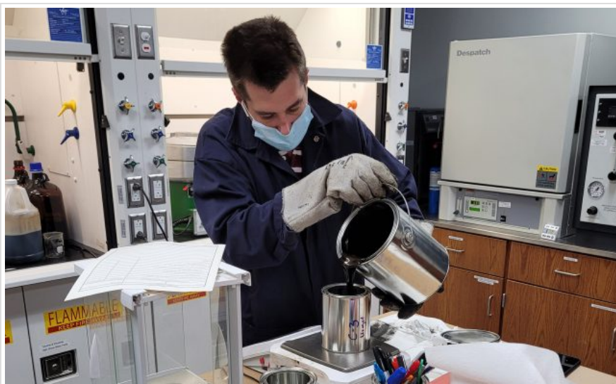
Joey Bonelli, a technician at the U.S. Army Engineer Research and Development Center, subsamples a graphene-enhanced asphalt binder. This binder has potential to increase asphalt strength and longevity. Photo courtesy U.S. Army Corps of Engineers
