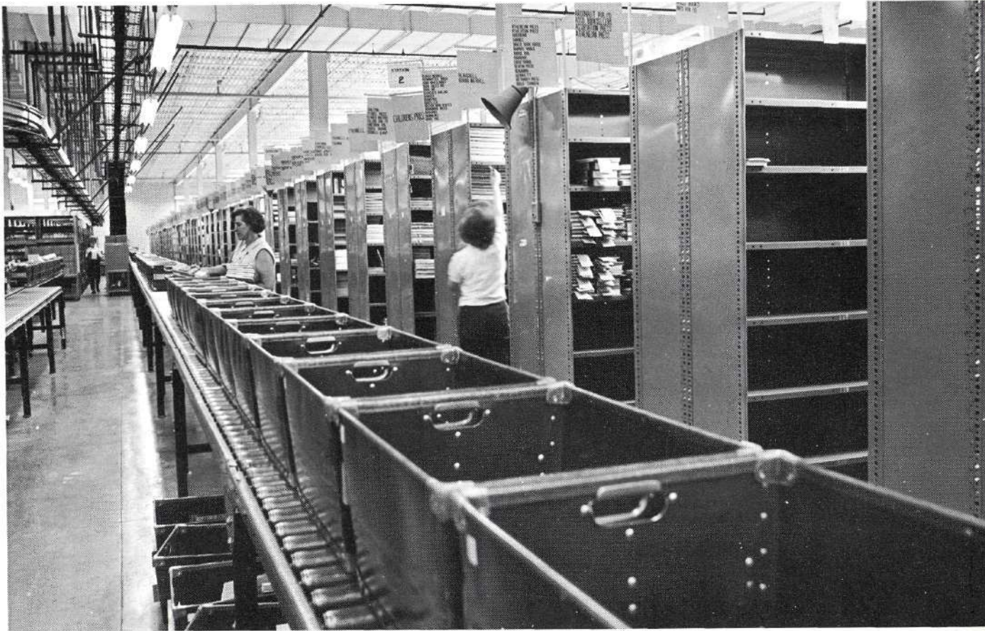
Picking lists are moved in bins that travel through the warehouse along a conveyor belt.
