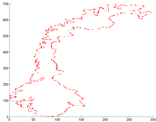
Figure 4.25: The original Norway image was randomly sampled to a set of 1086 surface points.
