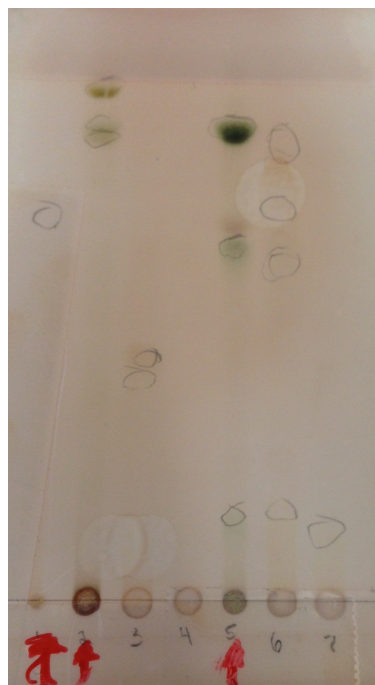
TLC: 90% DCM in Acetone (1: BC-C-2(13-32). 2: BC-C-2(1-5). 3:BC-C-2(10-13). 4: BC-C-3(1-5). 5: BC-C-3(6-9). 6: BC-C-3(10-12). 7: BC-C-3(13-29).)
