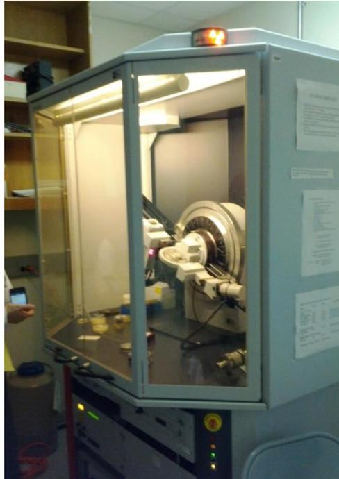
Figure 20: Bruker D8 Powder X-Ray Diffractometer at NCPA
