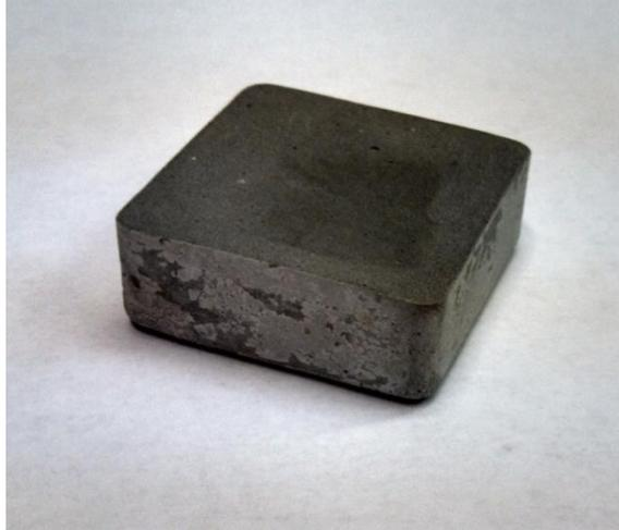
**Figure 37: Hardened Portland cement paste specimen ready for nanoindentation**
