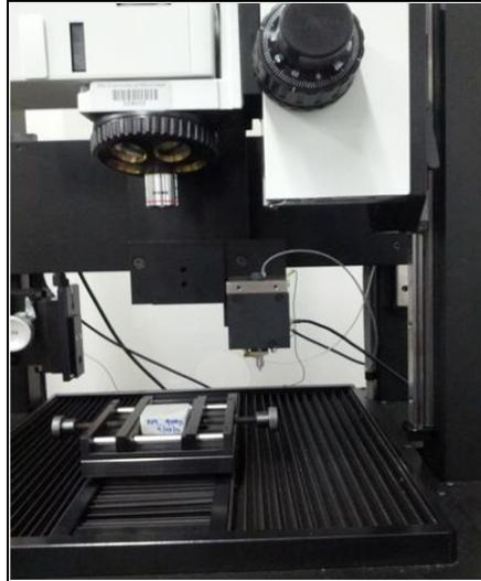
**Figure 2: Nanoindenter and Microscope**
