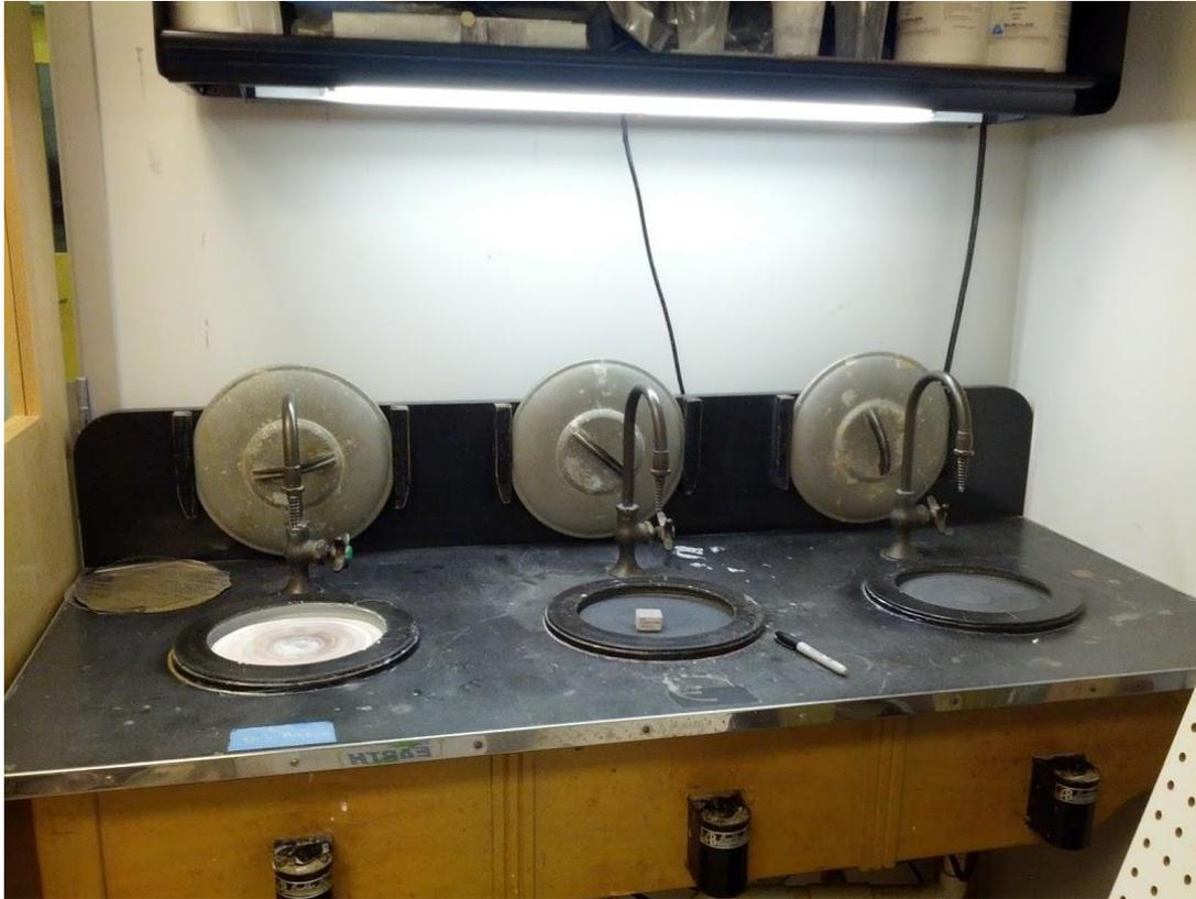
**Figure 23: Buehler Grinding/Polishing Table**
