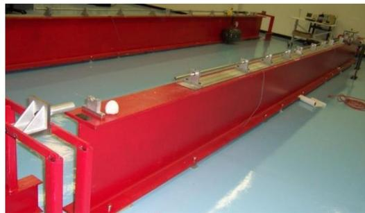
Figure 2. Hopkinson bar setup in the testing facility.
