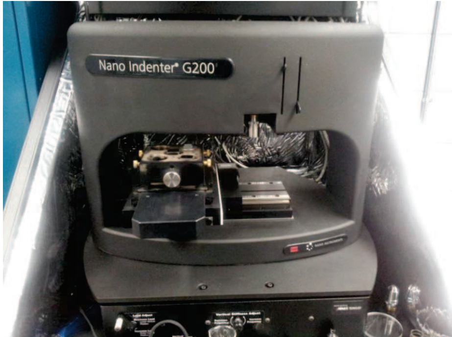
Figure 1.9 U9820A Agilent Nano Indenter G200 Used for Monotonic Analysis [20]
