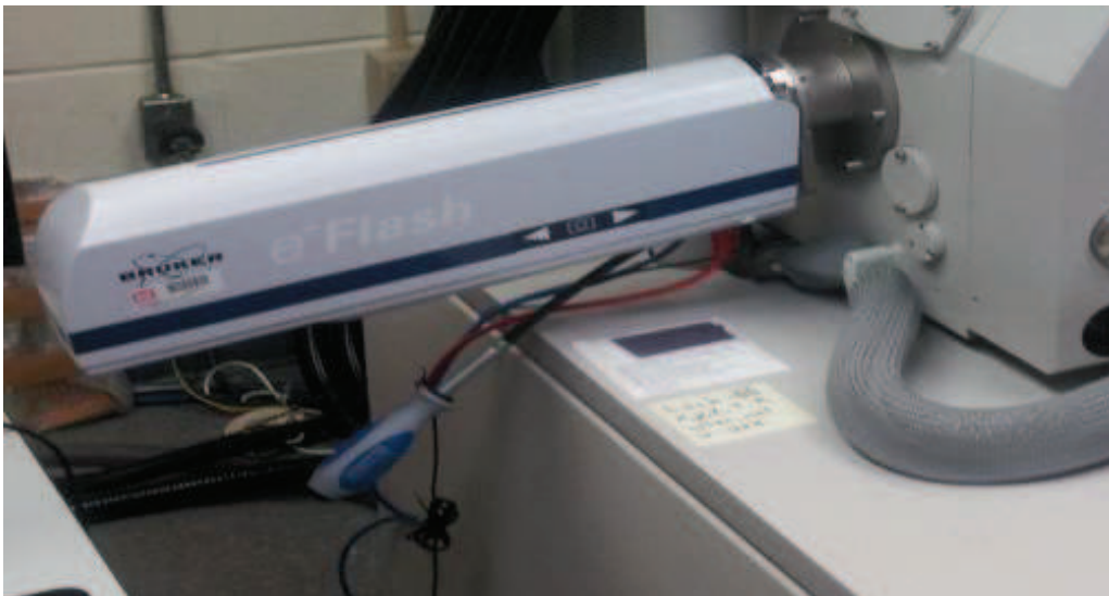
Figure 1.6 Bruker Quantax AXS Solid-State EDX Detector Energy Dispersive Spectroscopy Analysis Attachment [13]
