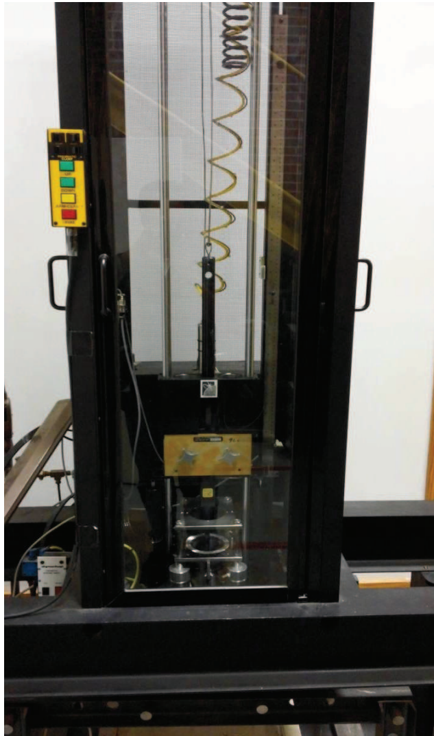
Figure 1.15 Dynatup 850 Low-Velocity Impact Testing Machine [25]
