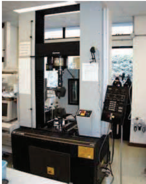
Figure 1.13 Instron 5980 Floor Model Universal Testing Systems Machine [23]
