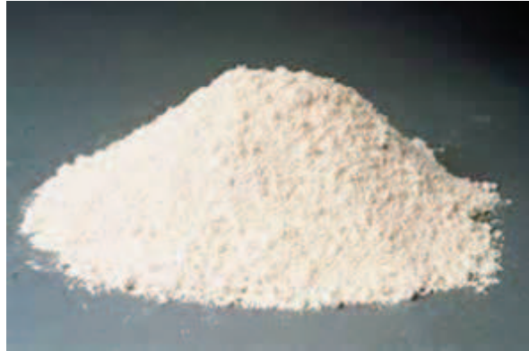
Figure 1.2 Unreacted Sample of Metakaolin [7]
