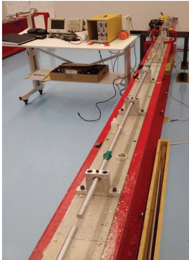
Figure 1.16 Split Hopkinson Pressure Bar at the University of Mississippi Blast and Impact Dynamics Laboratory
