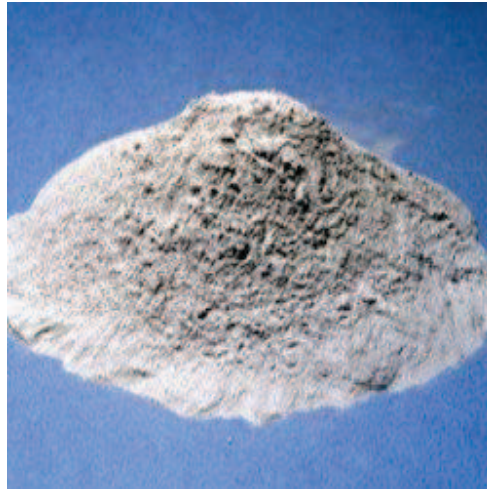
Figure 1.4 Typical Fly Ash Sample [8]
