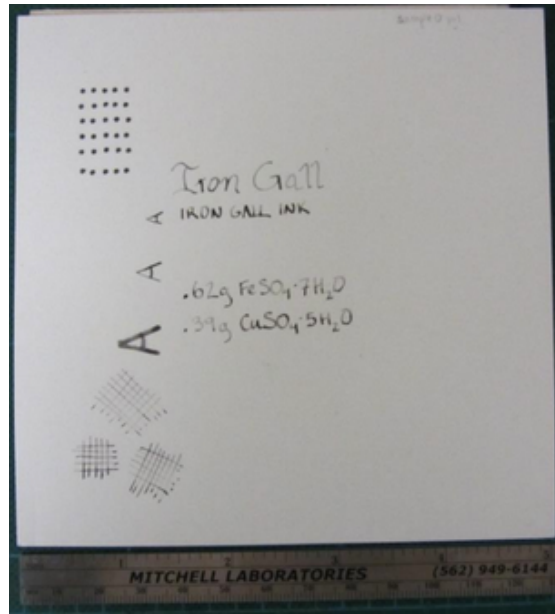
Figure 6.1: Prepared parchment sample for multispectral and Photoshop analysis.
