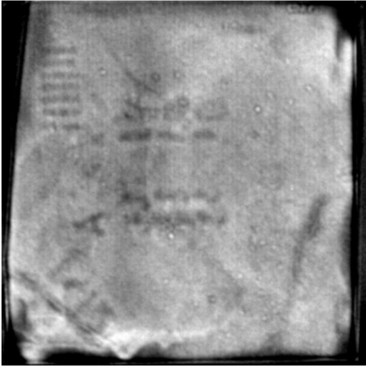
Figure 8.4: Thermographic image of ink on parchment at 2.37 seconds.
