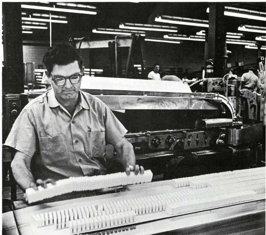
Delicately balancing a column of miniature Ivory soap bars by exerting just the right pressure, inspector checks them visually before putting them on wrapper line. At Ivorydale P&G packs Ivory, Camay, and Safeguard mini bars in the wrappers of several hotel and motel chains.
