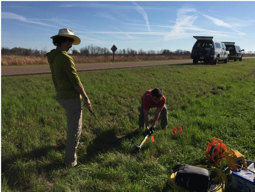
**Figure 21.** MASW survey near borehole TNA013.
