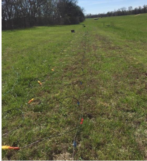
**Figure 22.** MASW survey near borehole TNA012.
