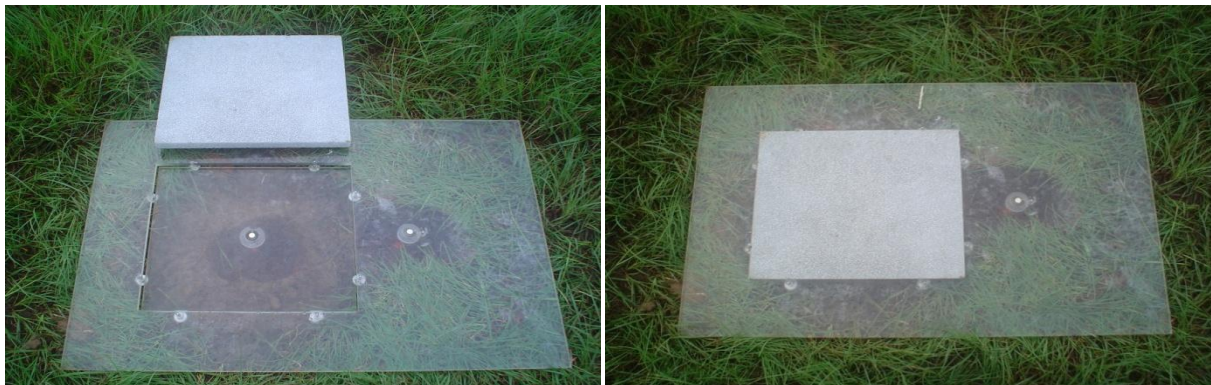
FIG. 4. Set up used by Yu 38 depicting the flush mounted microphones. The microphone on the right is left bare with its diaphragm flush with the plate. The microphone on the left covered by a sheet of foam, with the top of the foam set flush to the ground. (Images taken from Yu 36 )
