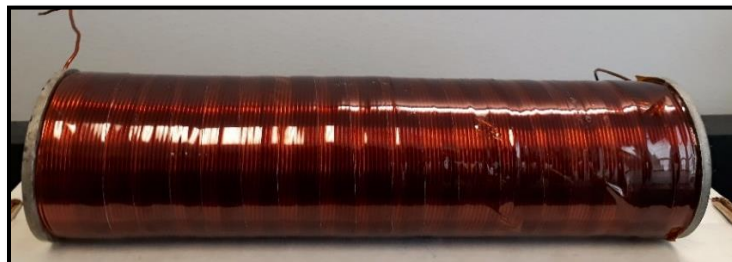
Figure 9 (Top) Large Solenoid built with 10 - gauge wire. (Bottom) Small solenoid built with 22- gauge wire
