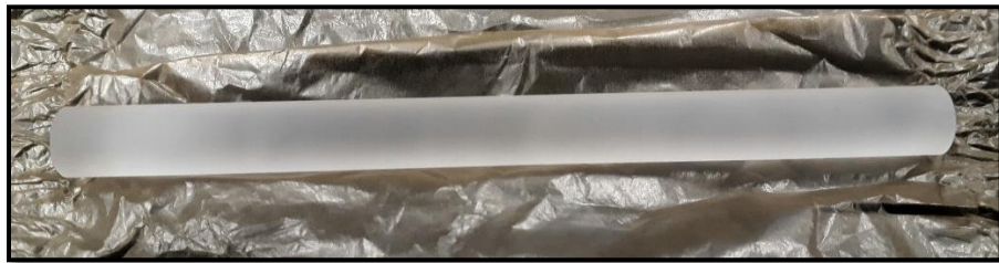
Figure 10 Corning 7980 quartz glass wrapped in black paper
