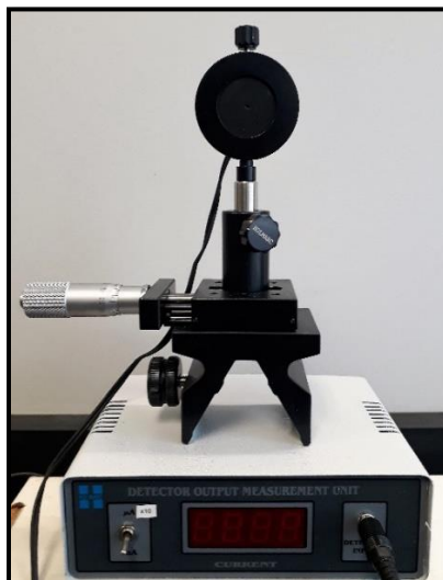
Figure 12 Pin-hole Photo Diode with output instrument
