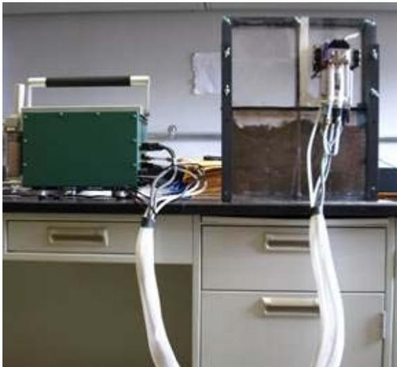
**Figure 1** – Photo exhibiting custom polycarbonate box gas chamber. The chamber is separated into two sections to seal the top of experimental mycocosms. One half of the chamber is used for CO<sub>2</sub> measurements and the other is sealed off entirely with closed cell foam (CCF) at base. The sensor head is attached to the center of the chamber wall and sealed with CCF. CCF is mounted
