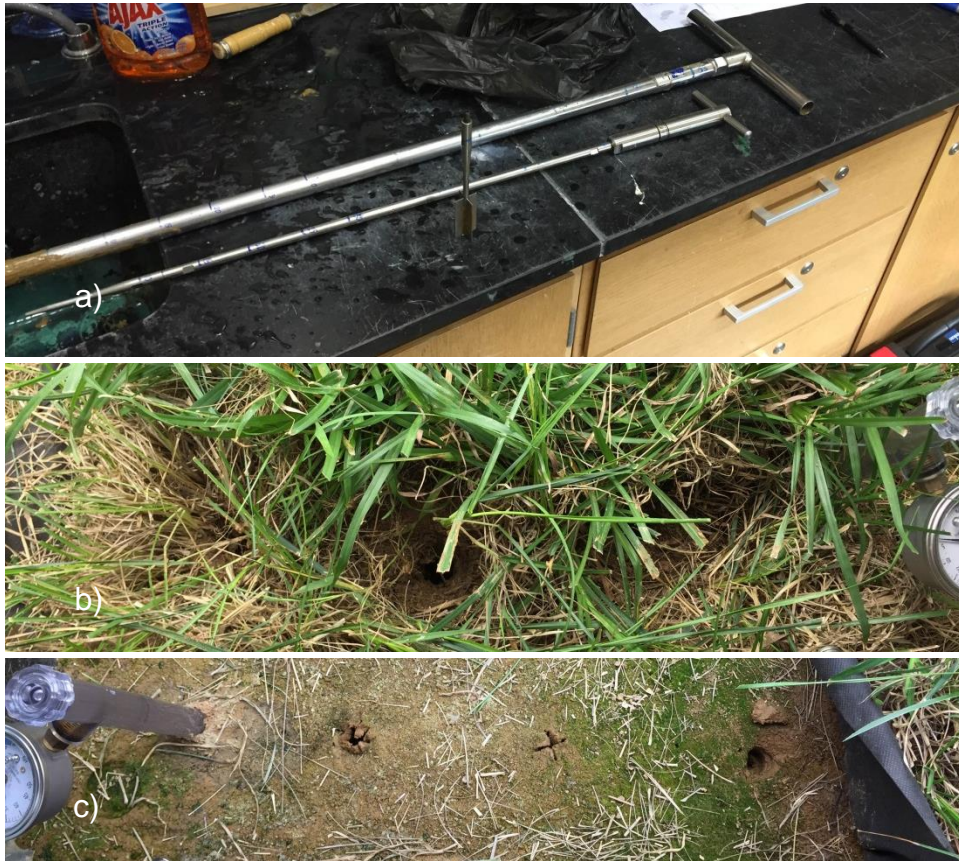
Figure 3.7 a) Shear vane tester, auger, and bore holes in b) Bahia grass and c) bare soil
