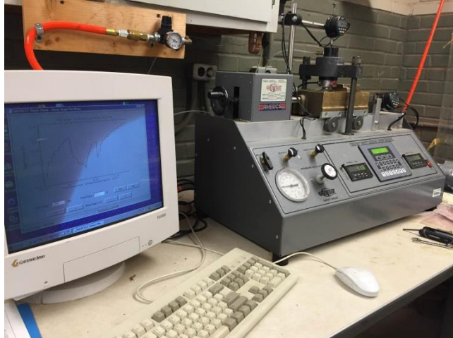
Figure 3.9 USDA NSL's direct shear test machine
