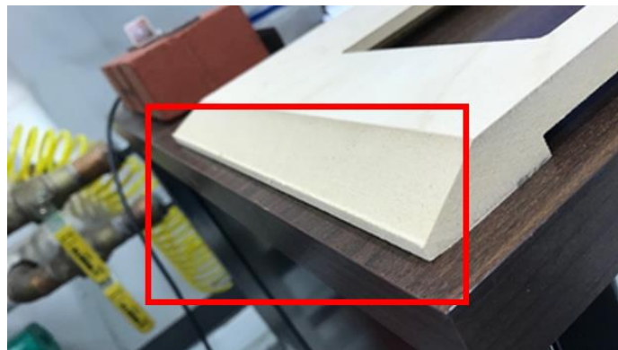
Figure 33 - Defect #3: Uneven Beveling
