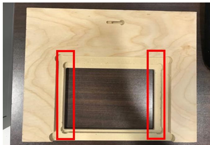
Figure 34 - Defect #3: Off-Center Front Opening
