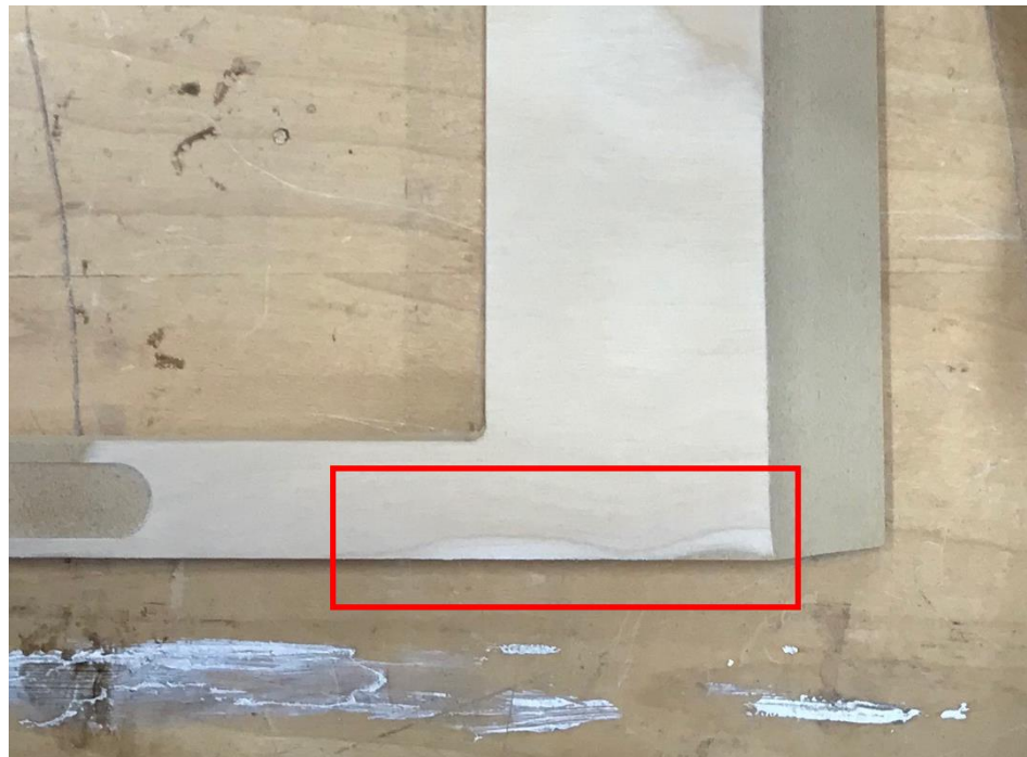
Figure 30 - Defect #1: Trial Frame (Power Sander)
