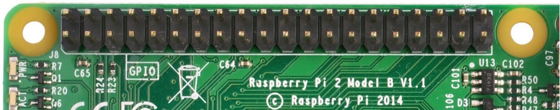
<figure 3 Raspberry pi GPIO Header block>--
