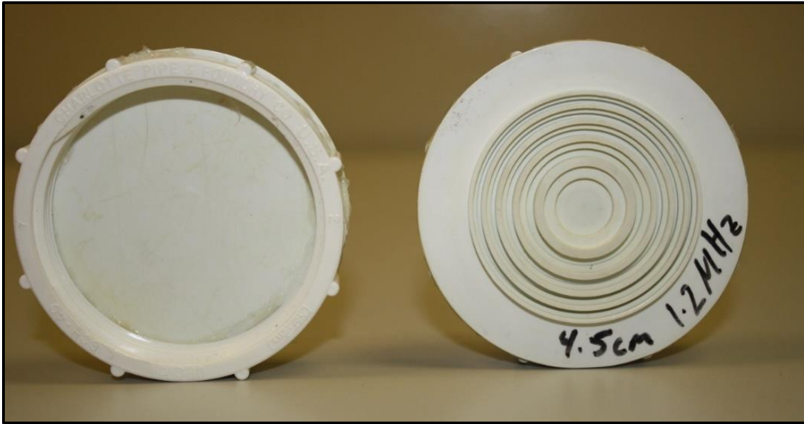
Figure 2.4: A photograph of Fresnel lens used to focus the ultrasound beam
