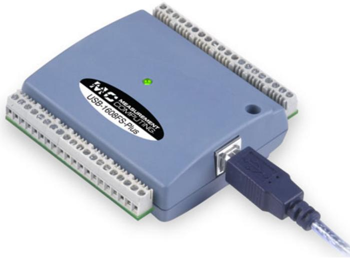
Figure 3.3: MCC USB-1608FS-Plus, non-OEM model
