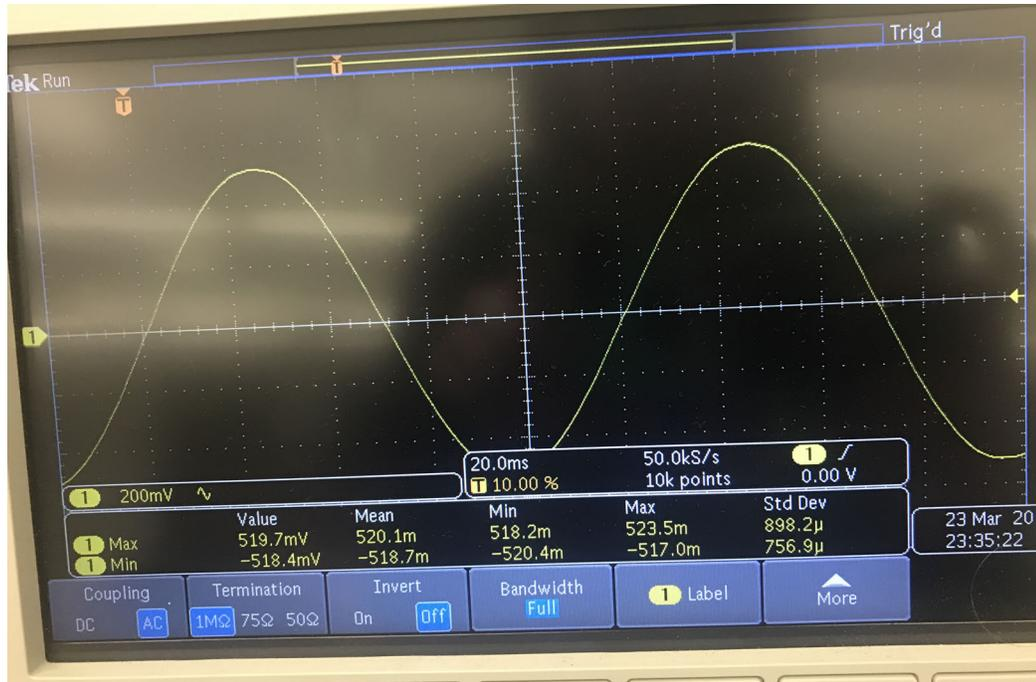
Figure 4.22: The output signal obtained from the instrumentation amplifier and high-pass filter circuitry – 10 Hz sinusoidal signal with amplitude of  $\pm 2$  V.
