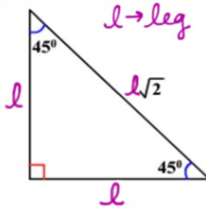
(We call  $45^\circ-45^\circ-90^\circ$  triangles a type of **special right triangle**.)
