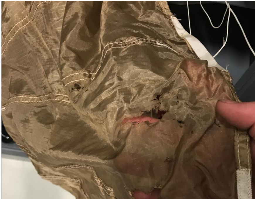
Figure 17: Damaged Drogue Parachute
