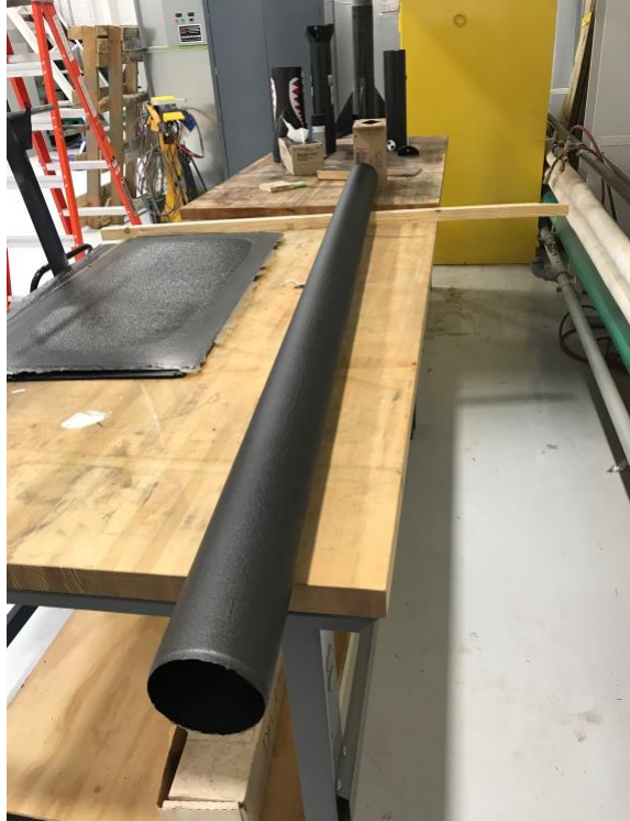
Figure 11: Post-Cured Body Tube and Stock Plates
