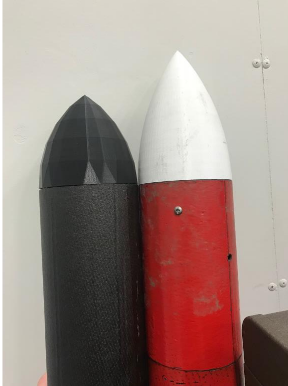
Figure 12: ABS and Ultem nosecones
