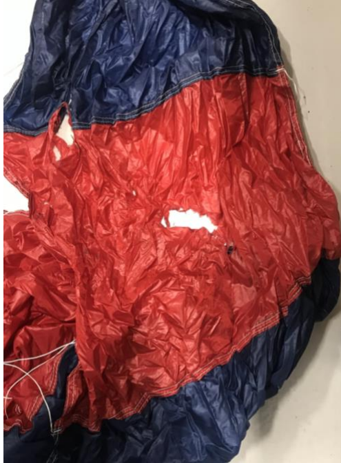
Figure 16: Damaged Main Parachute
