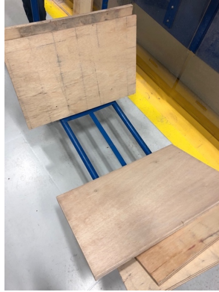
Figure 11: Pieces cut with Waterjet
