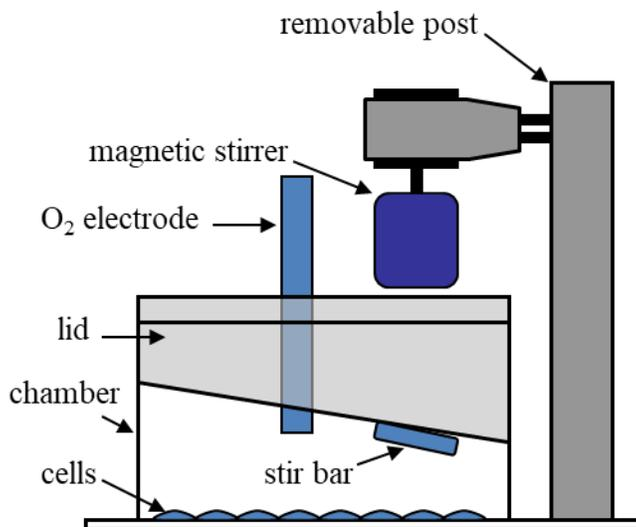
*Figure 2: Set up for respiration measurement. Shown are the cells plated at the bottom of chamber. A stir bar located in the media is being turned by a magnetic stirrer on the other side of the cell chamber lid. In the container is an O<sub>2</sub> electrode which measures the decreasing oxygen concentration of the buffer.*
