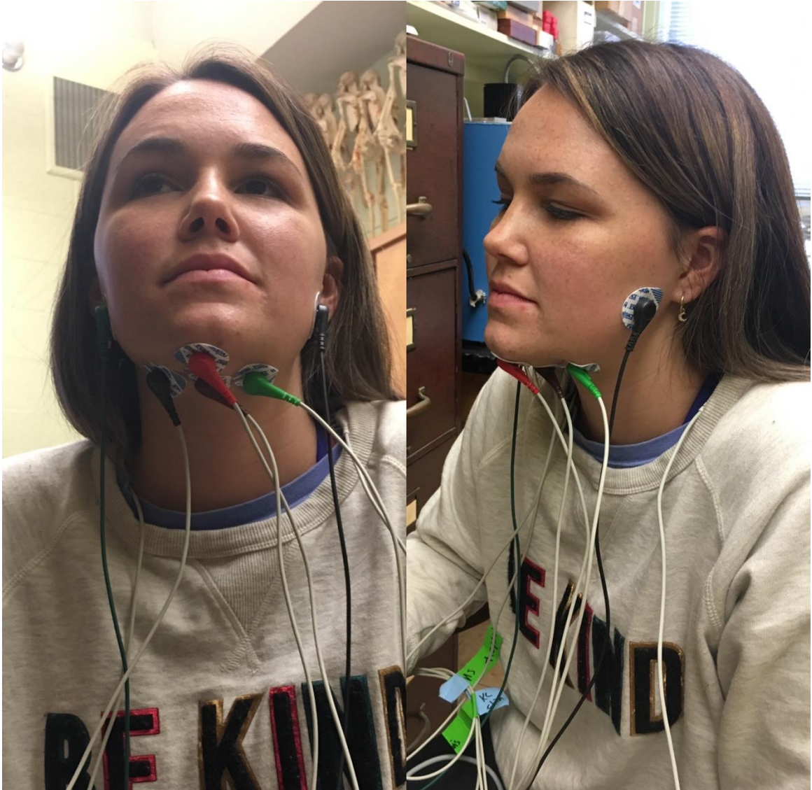
Figure 1: Electrode placement on participant includes four electrodes under the chin for measuring the contraction of the suprahyoid muscle (two on the anterior belly of digastric and two on the posterior belly of digastric), single electrodes on both masseter muscles, and single ground electrodes on both shoulders.
