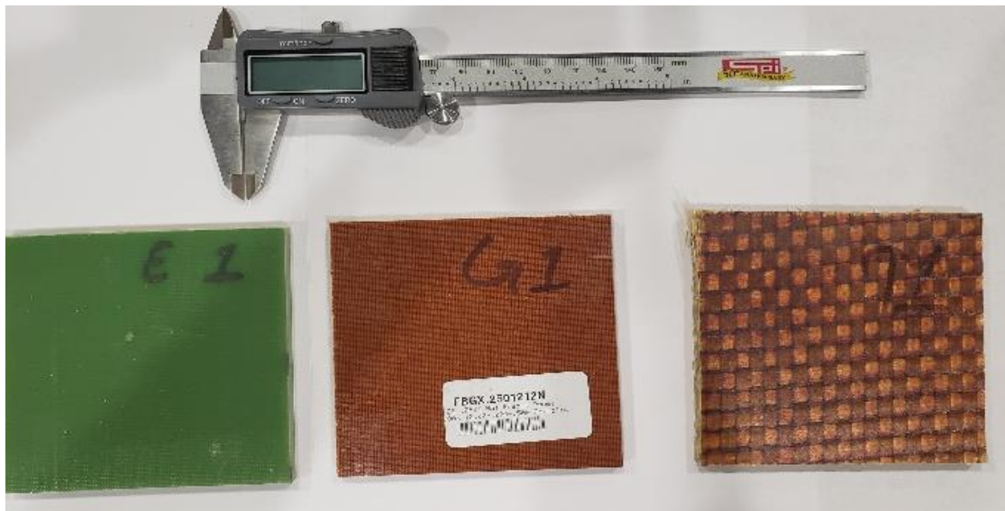
Fig 2. Sample Specimens for High Temperature G-11 (left), Economical Garolite (middle) and Impact Resistance Garolite (right)
