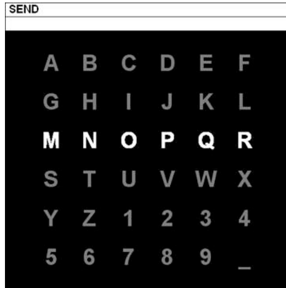
Figure 2.1: A P300 interface from the Brain-Computer Interface Laboratory at East Tennessee State University. This P300 system highlights the characters randomly, and waits for the P300 peak that appears in the user’s brain after she notices the wanted character being highlighted.
