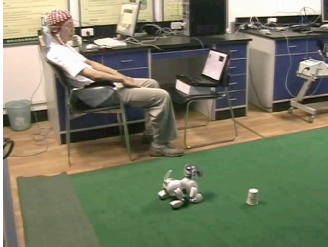
Figure 2.2: A motor-imagery system from the Tsinghua University. This system detects the activation in the user's motor cortex when the user simulates a given action in his brain, and translates this activity into commands to control the robot dog on the floor.
