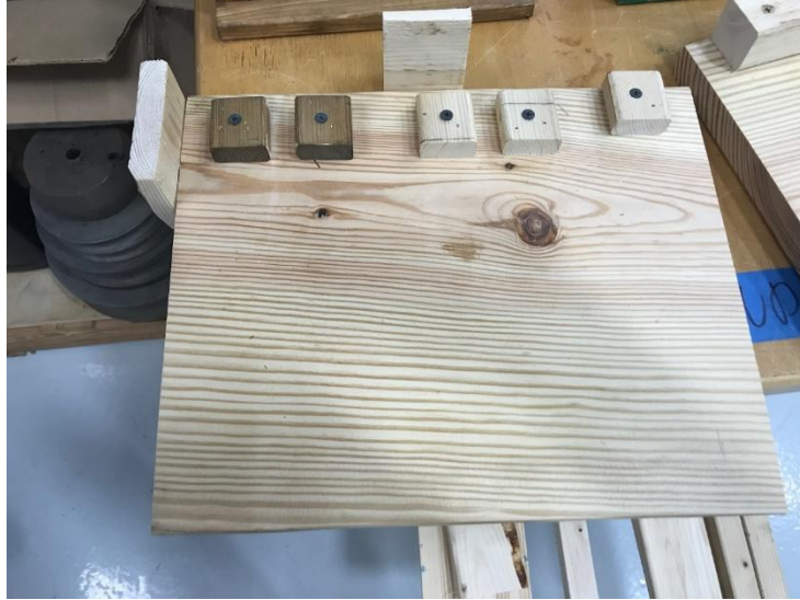
Figure 13: Jig 2 for the Connector and Controller Prongs
