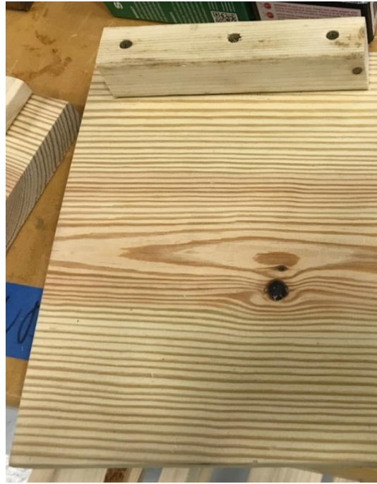
Figure 16: Jig 3 for Connector to Back Pillar and Base Connections
