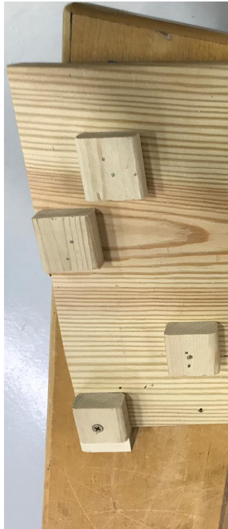
Figure 11: Jig 1 for the Connection of the Base and Back Pillar
