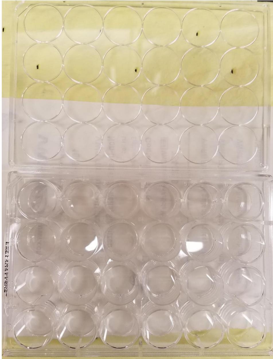
**Figure 6:** One of the trays used in this work. It is composed of a plastic 6 x 4 well system with a plastic cover. Note that the plastic cover is not the coverslip for the wells but it rather a protective shell to isolate the glass coverslips from damage.
