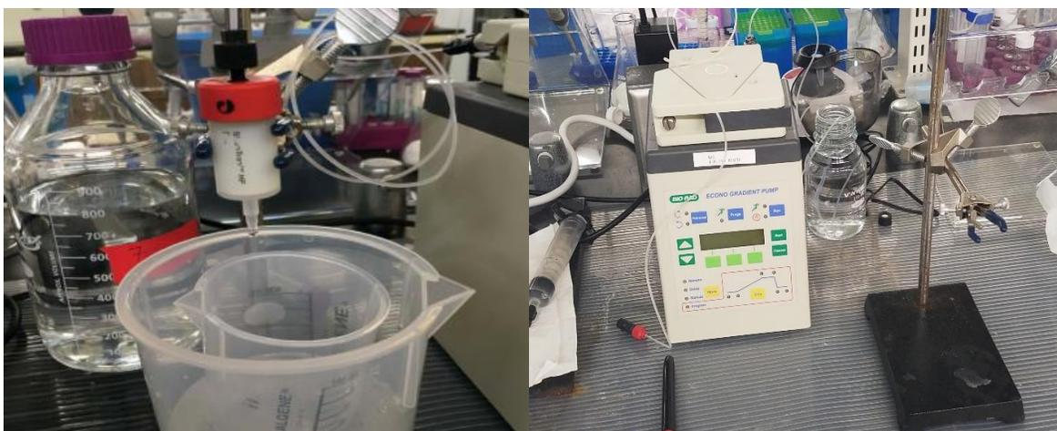
**Figure 17:** Strep-Trap affinity column (left) and the Econo gradient pump (right) used and associated setup
