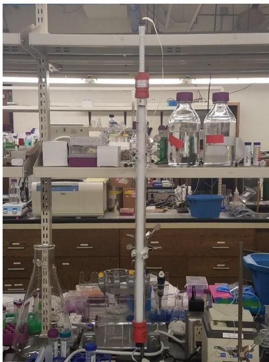
**Figure 18:** Size exclusion chromatography column used and associated setup
