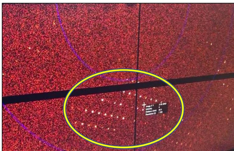
**Figure 23:** The diffraction pattern for apo-NBP crystals observed. The intense, luminous dots of lights within the yellow oval correspond to relevant diffracted x-rays
