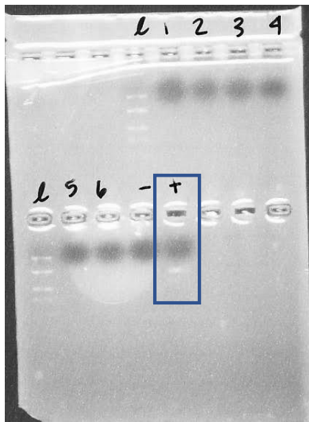
Fig. 1 A scanned photo of an electrophoresis gel image with a faint band on the positive control.
