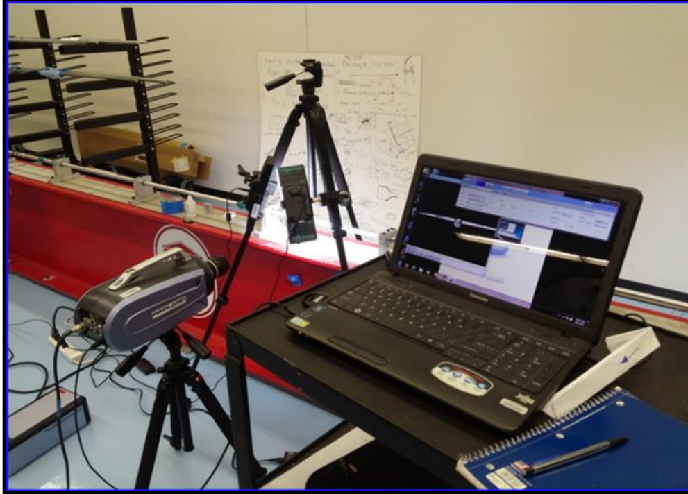
Figure 5: SHPB and High-Speed Video Setup
