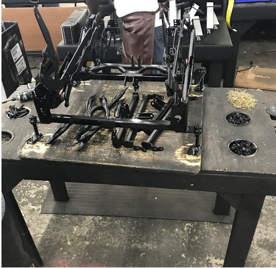
Photo 2: Metal Framed Jig, top view
