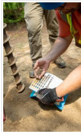
Lance Yarbrough, UM associate professor of geology and geological engineering, uses a Munsell chart to record the correct color of clays observed in the field. Photo by Kevin Bain/Ole Miss Digital Imaging Services
