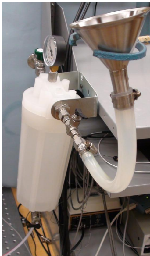
Figure 7 : Fill reservoir used to load ultrapure water into sphere loop. The reservoir was constructed with ultrapure polypropylene, and all other fittings and tubing were stainless steel, PTFE, or ultrapure Tygon®.
