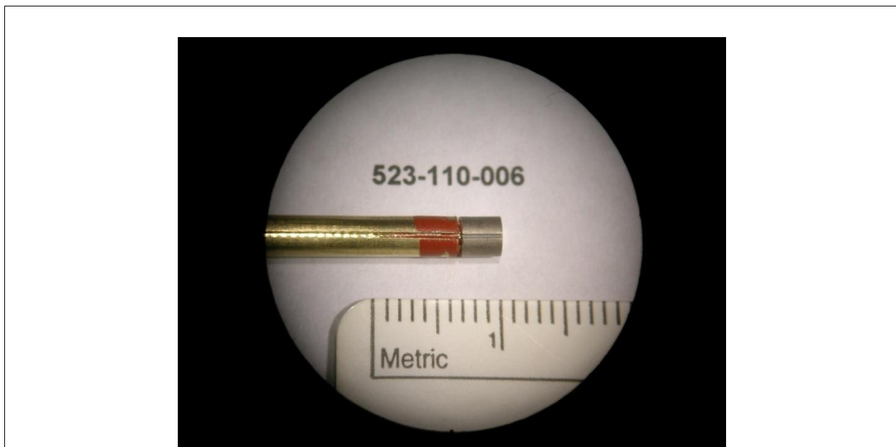
Figure 57: Photograph of the hydrophone mount after assembly of the PZT element. (S/N 523-110-006)
