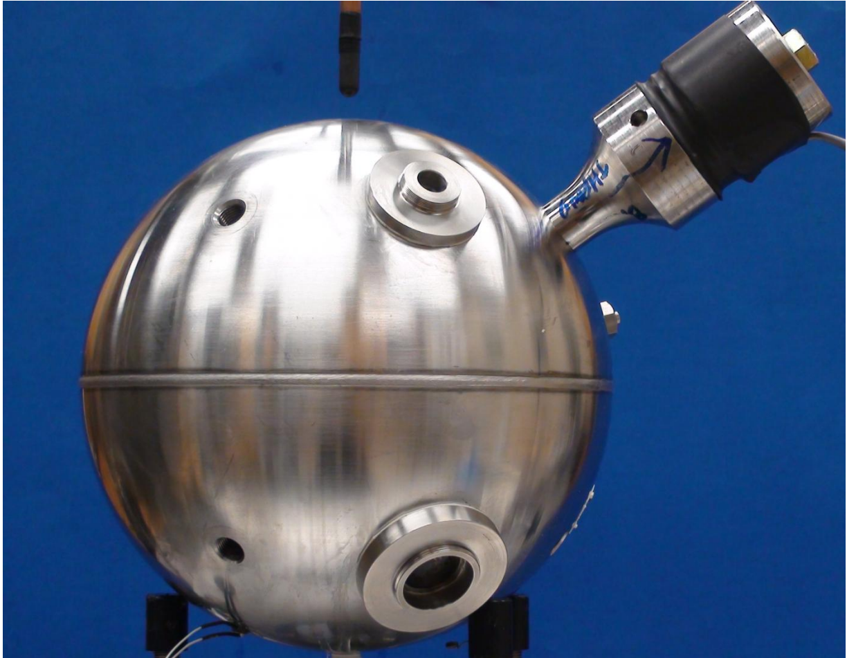
Figure 9 : Photograph of spherical resonator used for reported results. The sphere was 9.5” outer diameter, 0.75” thick with a total volume of approximately 4.4 L. The material was type 17-4 stainless steel.
