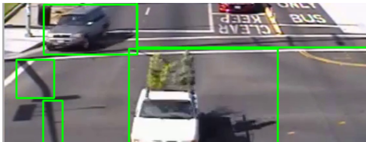
Figure 3.3: Object Detection based on Consecutive Frame Difference
