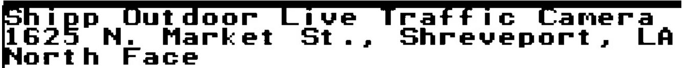
Figure 2.4: Simple Binary Inverse Thresholding
