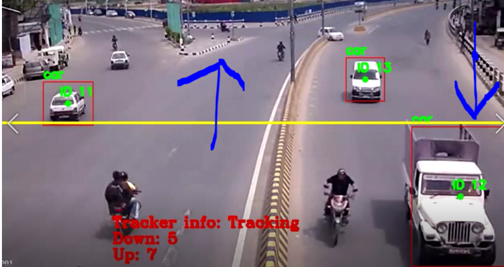
Figure 5.2: Counting algorithm. Yellow represents the reference line (Rosebrock, 2020). SSD Mobilenet v2 was used for detection.
