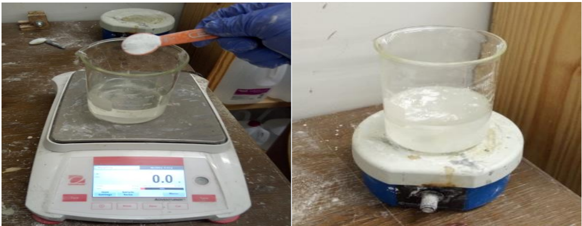
(b) Dissolving the boric acid by the thermix stirrer with a speed of 300 RPM for 15 minutes
