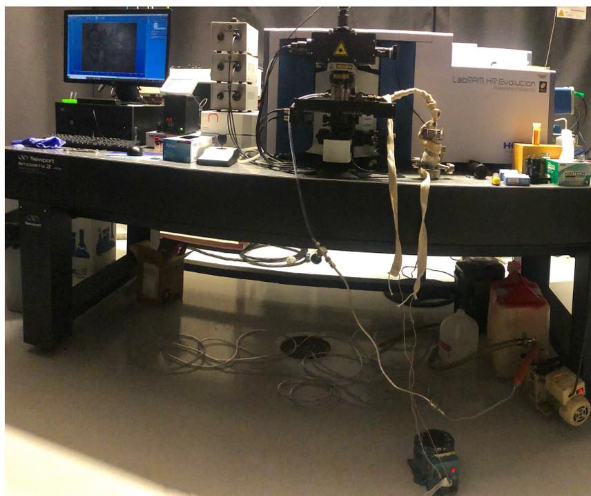
**Figure 4.2.1:** Image of Custom Raman spectroscopy setup
