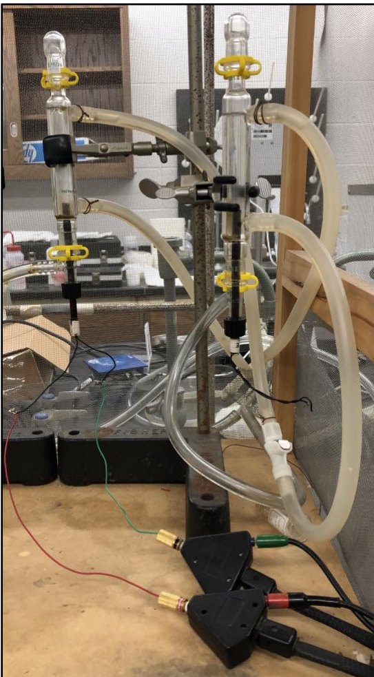
Figure 11. Setup for conductivity trials with custom built electrodes in a Faraday cage.
