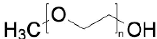
Figure 5. General structure of the polyethylene glycol monomethyl ether. Monomethyl polyethylene glycol (MW = 164 g/mol) has a n-value of 3.
