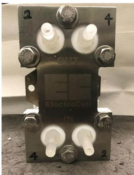
**Figure 3-2:** Front view of ElectroCell system showing inlet and outlet ports
