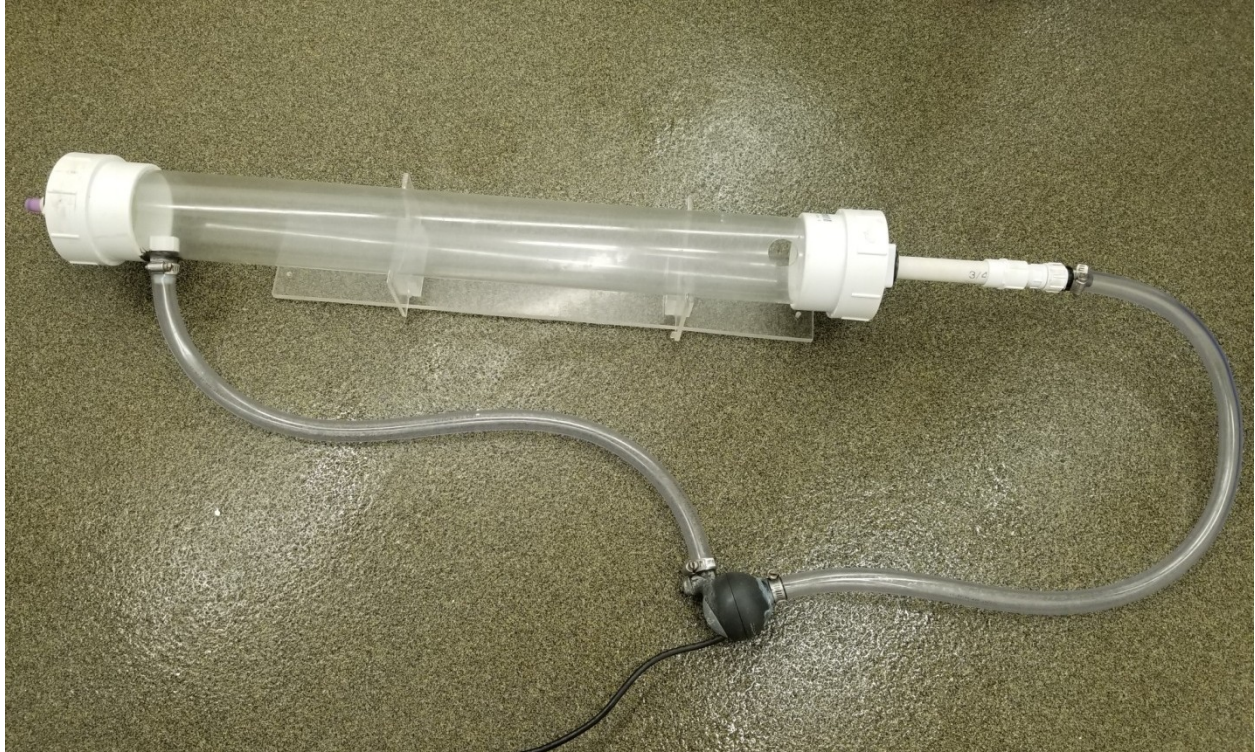
Figure 13. The respiration chamber constructed and utilized for sedation experiments with C. plagiosum .
